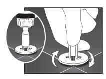
When four tiles intersect (or two tiles when using EDGE spacer) and with mortar still fresh, turn spindle clockwise until tiles are flush.
