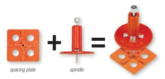
The spacing plate and spindle hold the tile in position, creating precise intersections and perfect lines. Turn the spindle clockwise until tiles are aligned and flush. Remove spindle when adhesive is dry.
