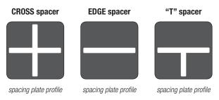
Use **CROSS** and **EDGE** spacers for standard, grid tile patterns and **T** and **EDGE** spacers for offset patterns.
