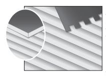
Spread tile mortar onto tile-ready substrate using a trowel size appropriate for the specific tile format. The use of a levelling system requires use of a larger trowel notch than usual, for this reason it is suggested that a minimum 10mm or
