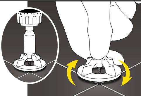
When four tiles intersect (or two tiles when using the EDGE spacing plate) and with mortar still fresh, turn spindle clockwise until tiles are flush.
