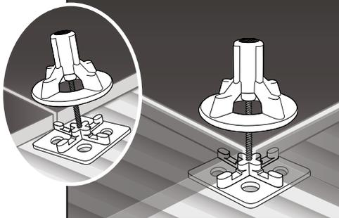
Thread spindle into spacing plate.
