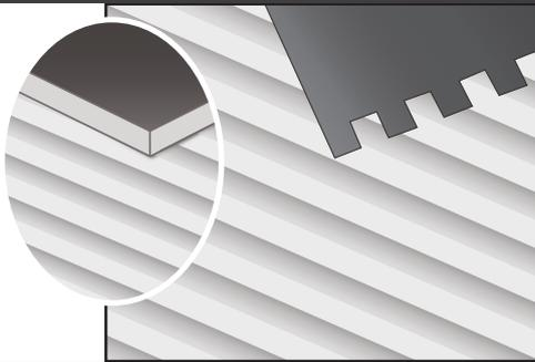
Spread tile mortar onto tile-ready substrate using a trowel size appropriate for the specific tile format. The use of a leveling system requires use of a larger trowel notch than usual, for this reason it is suggested that a minimum 10mm or 3/8in square notch trowel is used.
