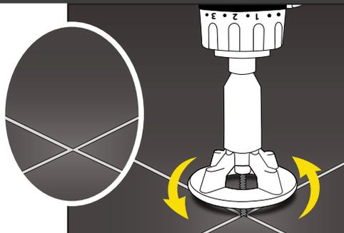
Once mortar has cured according to manufacturer's guidelines, remove the spindle by turning counter clockwise.
